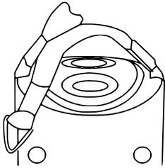
Open the battery case cover on the rear side of the device to insert two batteries (1,5 V AA batteries, not included).
