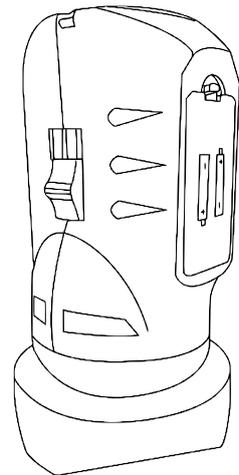
Switch off the construction laser when it is not in use or whenever you cannot observe it. Secure the device by using the lock bar on the side.
