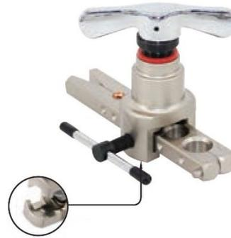
5. Tighten the knob clockwise. To make the pipe smooth, turn another 2–3 turns.
