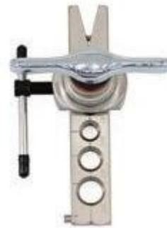
6. To remove the pipe, turn the knob upwards in anti-clockwise direction. Do not tighten the T-handle until the knob is not in its uppermost position. Remove the pipe.
