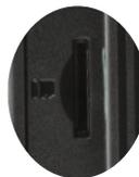
Note: TF card is only used for storage and playback of driving recorder. Music playing software cannot read this card slot.
