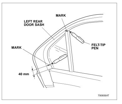
7. Temporarily position the two frame clips on the door sash aligning the end of the frame clips with the marks you made in step 4 and attach the pieces of masking tape as shown.
