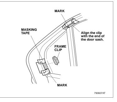
9. Apply primer to the parts of the door sash enclosed with the masking tapes and let it dry thoroughly.
