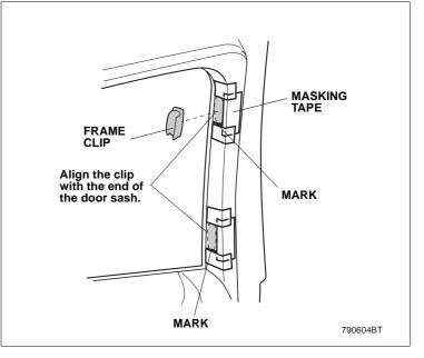
8. Temporarily position the frame clips on the door sash aligning the end of the frame clips with the marks you made in step 6 and attach the pieces of masking tape as shown.
