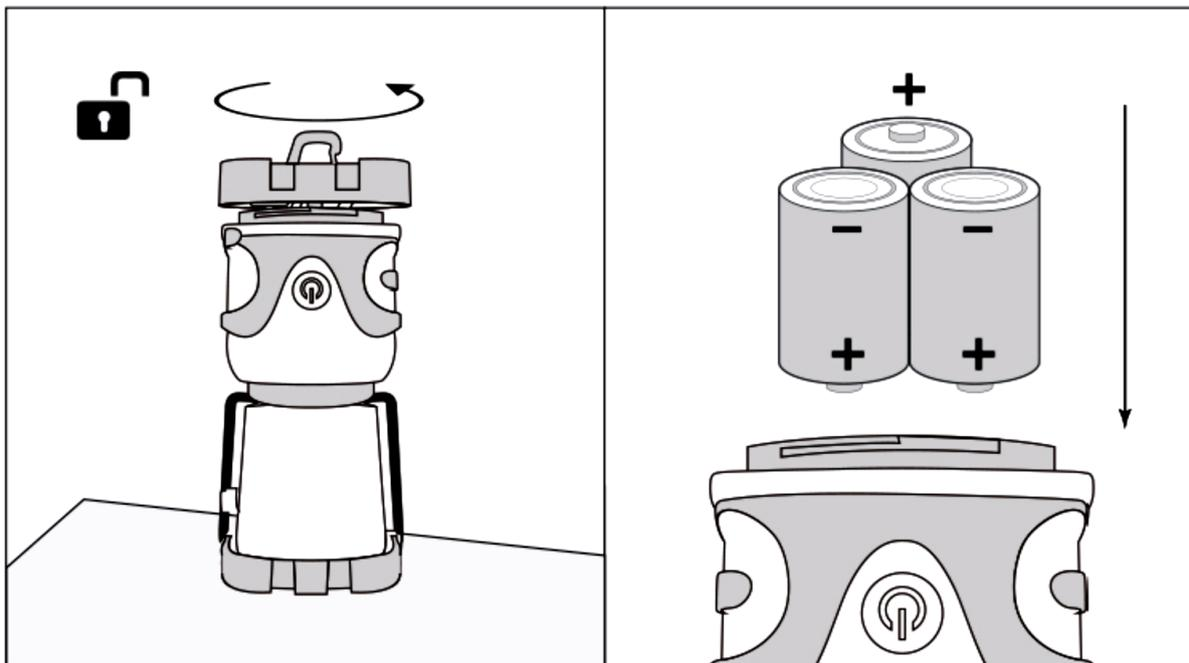
1. Turn the lamp upside down and unlock the base by turning it. 2. Insert the batteries in the correct direction. **Caution:** Do not use rechargeable batteries!
