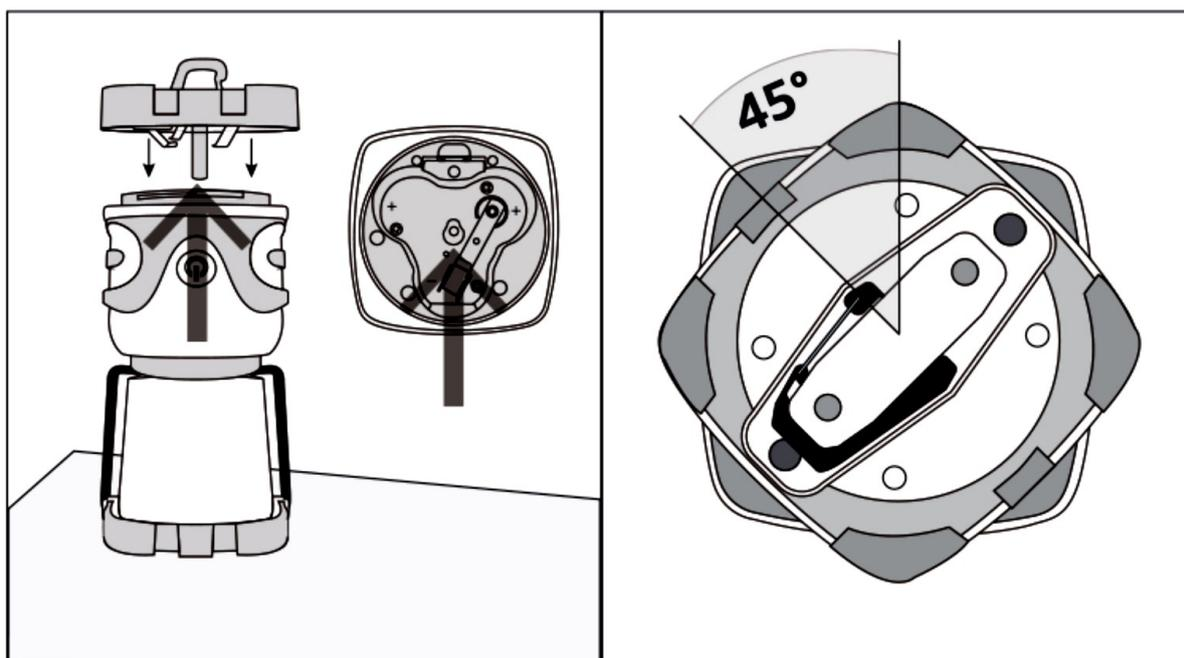
3. Replace the base while making sure that the pin is at the correct position (see arrow). 4. Re-lock the base by turning it.
