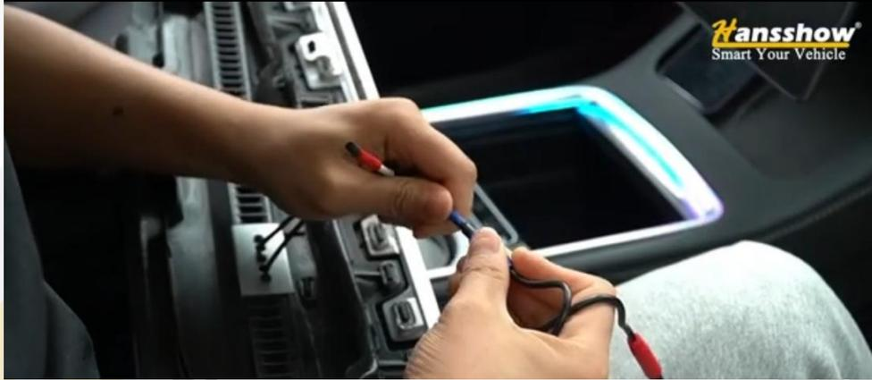
9. Connect the red and blue wires together.
