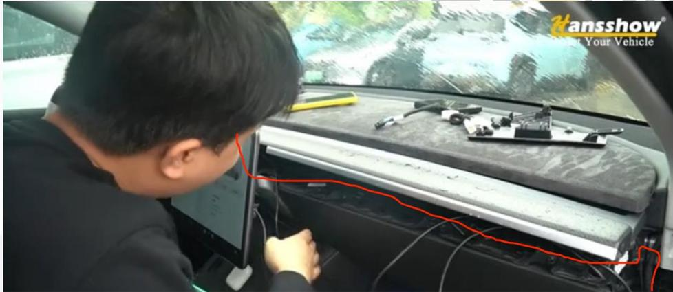
10. Run the wire harness along the center console, being careful not to let it be compressed by any clips, and try to make it as tidy as possible (you can use vinegar adhesive tape to fix it firmly). Finally, restore the center console and other panels to complete the installation.
