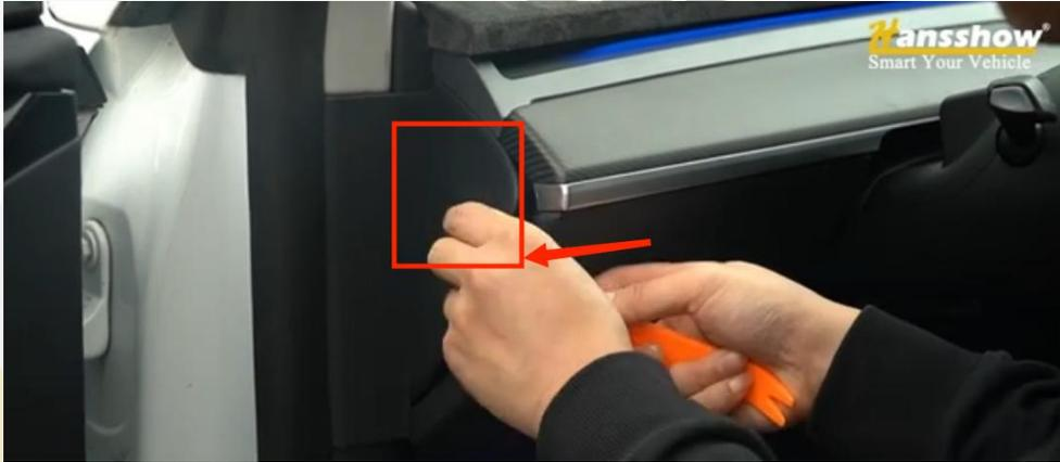
1. Use a pry bar to pry open the left and right small side panels.
