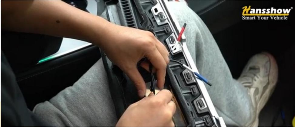
5. Thread the wires of the mini display through the metal gasket and fix it in place with a screw.
