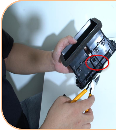
8. Cut off the middle clip at the top of the A/C outlet.
