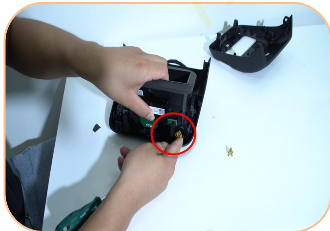
11. Install the clips onto the screen panel
