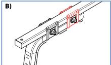
**CLAMP SET FOR RAINGUTTER FOOT** For installing roof rack onto raingutter foot (1 set each 2 feet)
