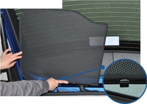
INSERT CLIPS BEHIND INTERIOR TRIM
