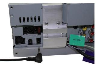
4. Connect the 14 way molex connector, the car display connector (from the vehicle) and the chime retention box to the interface.
